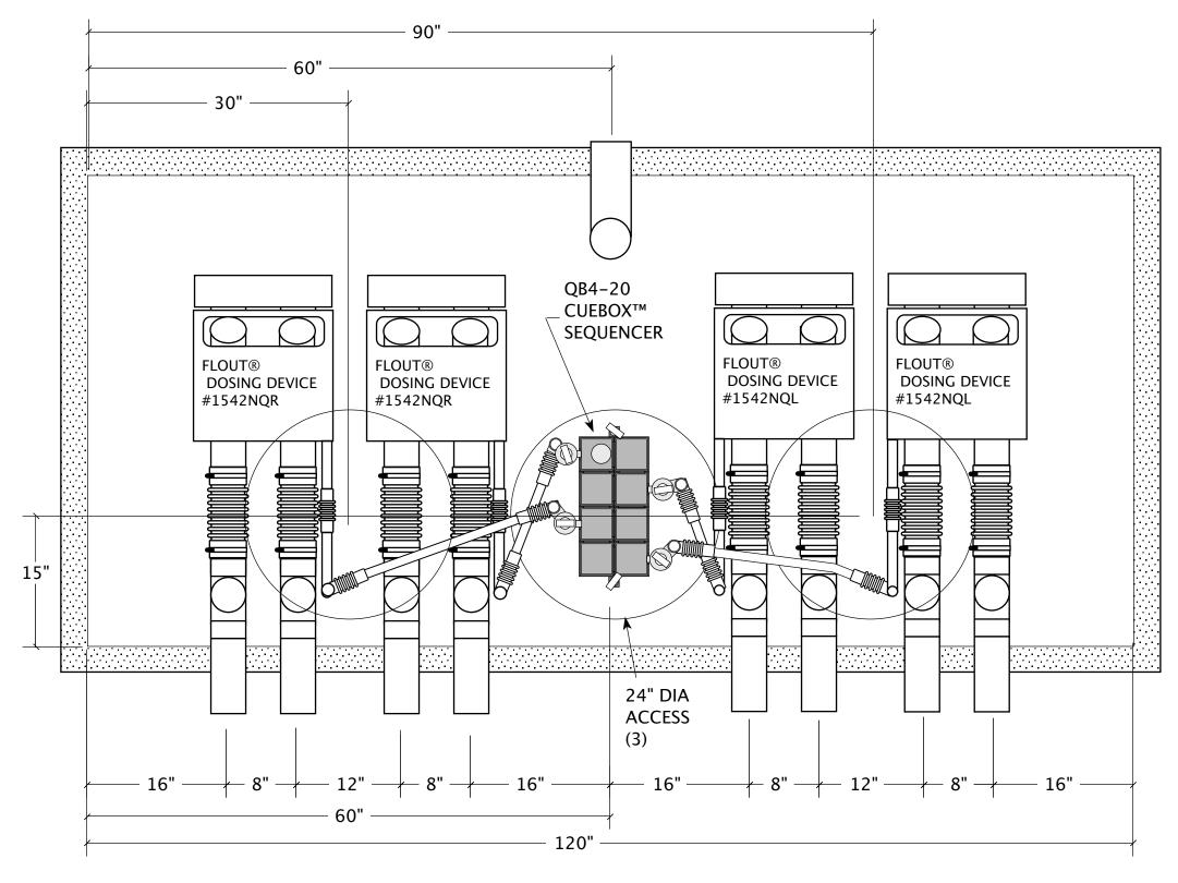
A PROPOSED DOSING CHAMBER WITH FOUR FLOUT® DOSING DEVICES EACH WITH TWO 4 INCH DIAMETER OUTLETS. DOSING SEQUENCE CONTROLLED BY A CUEBOX™ SEQUENCER. 15 INCH DRAWDOWN.
